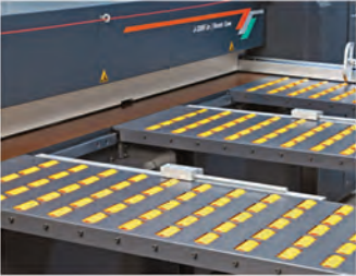
Back Support rollers for easy & smooth movement
