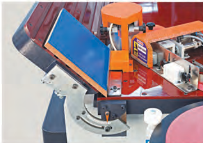
Hylum surface working table with 45° tilt
