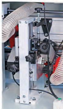
Fine Trimming with Diamond Cutters
