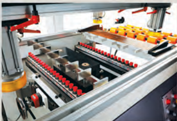
For vertical boring application. Both heads work parallel vertically
