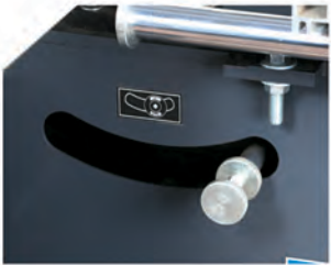
Scoring saw precision lever mechanism
