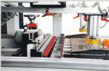
Horizontal & vertical Boring
