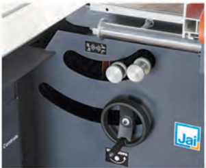
Scoring saw precision lever mechanism
