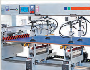
Support rollers have 4 reference stops for lengthy workpiece
