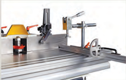
Mitre Gauge with Clamping
