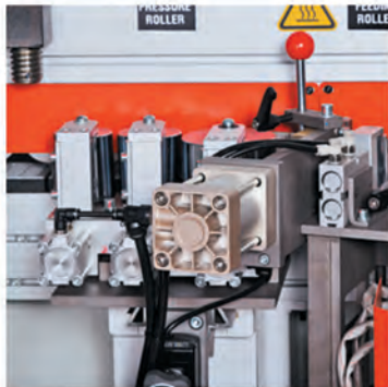
3 Pressure Roller with Scraper
