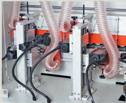
Rough Trimming & Fine Trimming with Diamond Cutters
