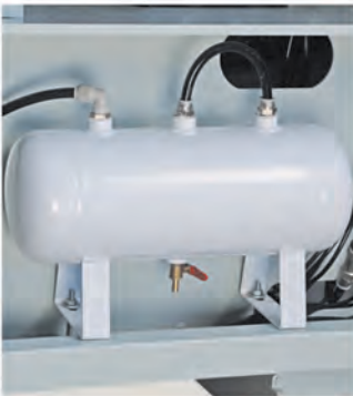
Safety Air Tank for non-dropping of air during process
