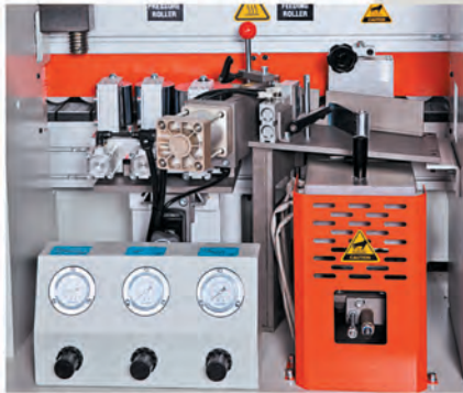
3 Pressure Roller with Scraper
