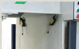
Dual limit switch to control the pressing of work piece
