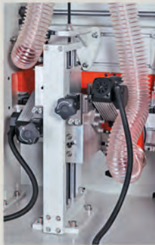
Fine Trimming with Diamond Cutters
