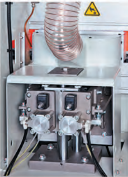
Pre - Milling with Diamond Cutters
