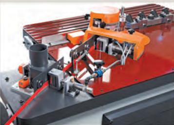
Pneumatic cutting device with 45° Edge tape grooving for 45° panel
