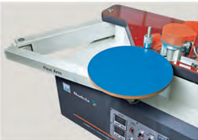
Flexible arm for easy movement of curved panels.
