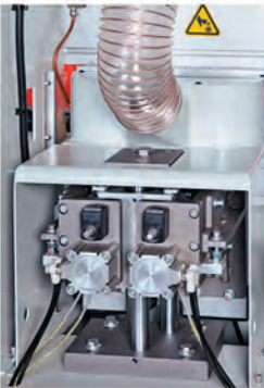
Pre - Milling with Diamond Cutters
