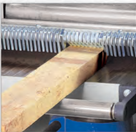
Anti kick-back system to avoid backsliding
