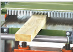
Anti kick-back System to avoid back sliding
