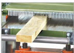
Anti kick-back System to avoid back sliding
